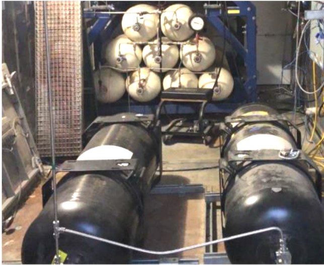
Smart dispenser components being tested with storage.
