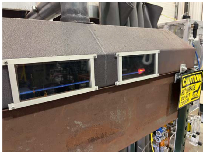
Ribbon burner test setup in laboratory
