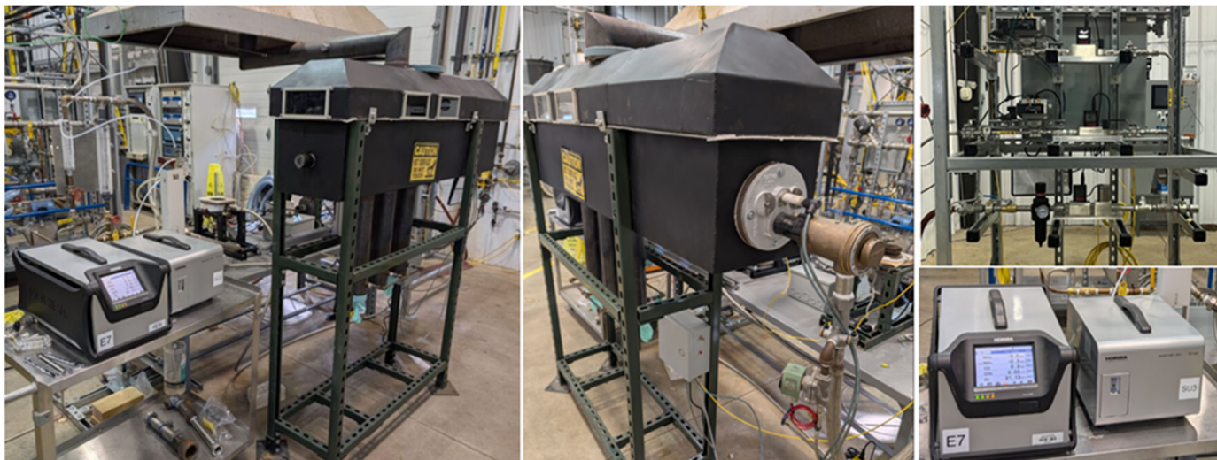
Photograph of the burner test-stand (clockwise from left: overall view of the test rig, test stand, fuel and air metering equipment, sampling equipment)
