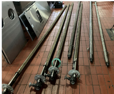
Combi-burners, zone 5 replacement and interior re-firing
