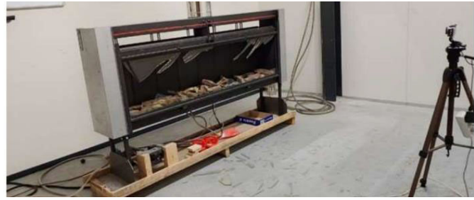
Catastrophic gas fireplace failure during delayed-ignition tests with 30% H2 blends, otherwise not seen with pure natural gas (Image credit: www.thyga-project.eu )
