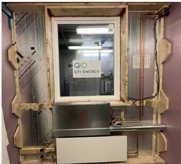
Hydronic Shell envelope/mechanical panel
