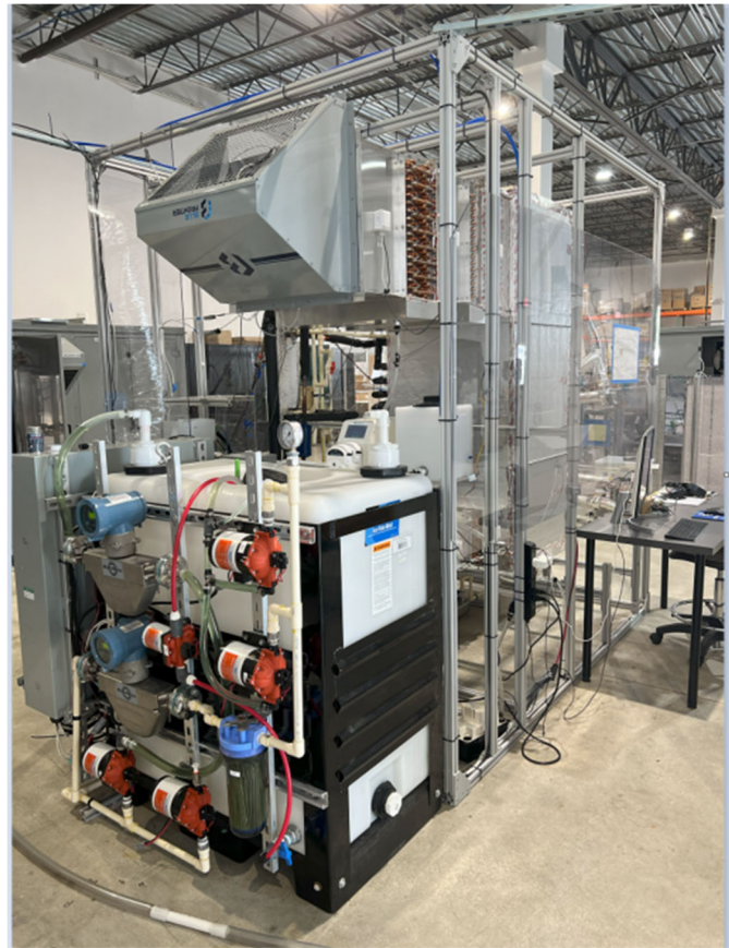
Blue Frontier regenerator section to be tested with an mCHP thermal load
