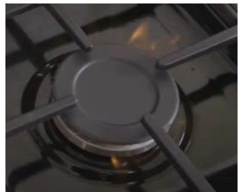
Nearly Invisible Hydrogen Flames: North America Hydrogen Hut Field Testing on a Cooktop Burner (Left) and 100% Hydrogen Cooktop Burner Flame from HY Grove, UK (Right).
