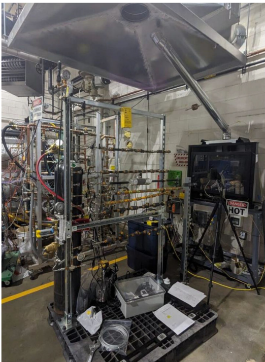
Leakage test apparatus during shakedown tests.
