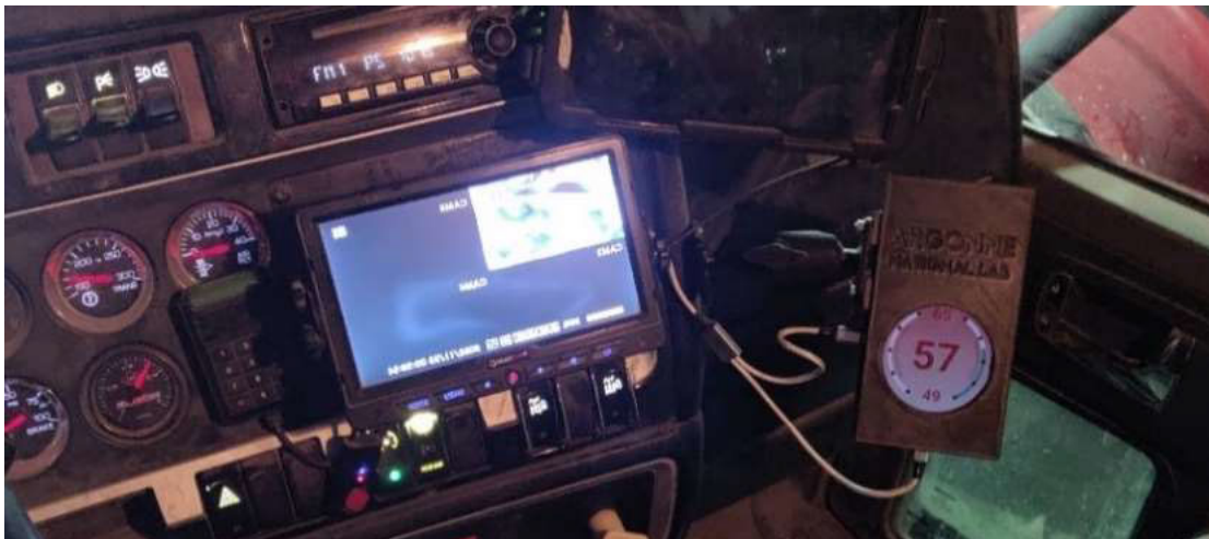
First installation of the prototype next generation NGV fuel gauge and driver information system in a ready-mix concrete delivery truck
