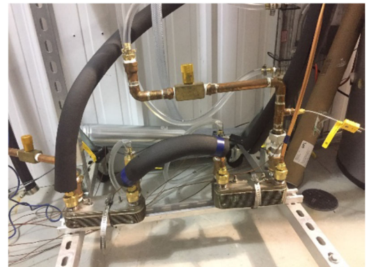
LG 25MBH heat pump with evaporator outside (left), tankless water heater with condenser heat exchanger (middle), condenser plate heat exchanger (right)
