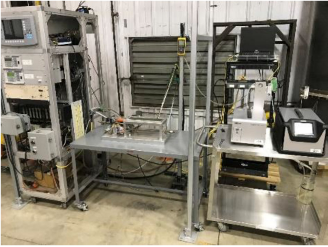
Test setup used to perform IR burner evaluation with Solaronics burner installed on the test-stand
