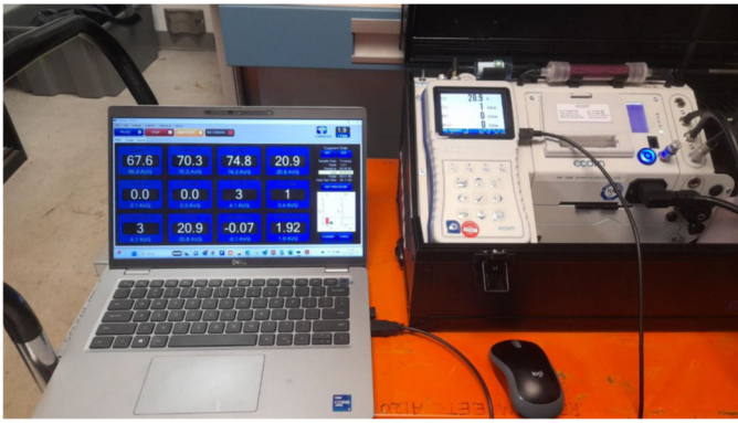
Electrochemical sensor - ECOM J2KN analyzer with a hydrogen sensor
