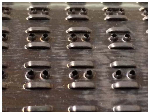
Figure 15. Burner Combustion Surface
