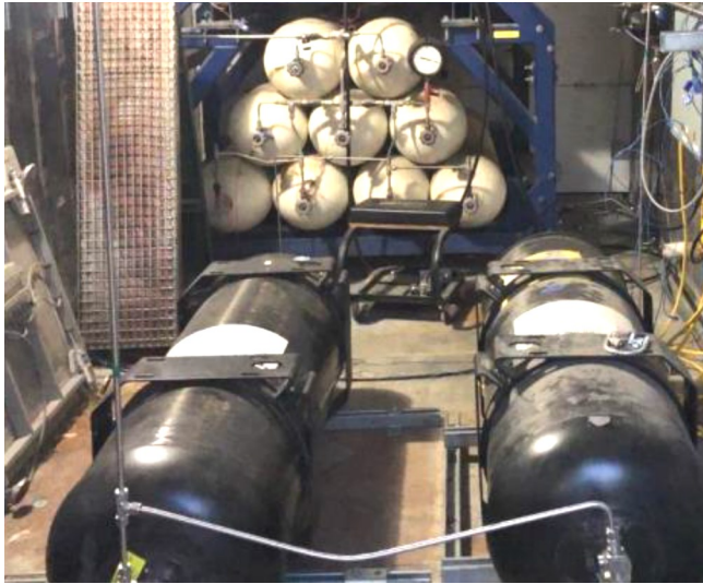
Smart dispenser components being tested with storage.
