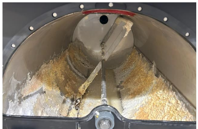
Interior of reaction chamber after operating unit for a few hours with ~25 kg of caustic potash
