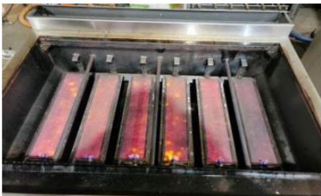
Burner assembly with multiple IR burners designed for host site.
