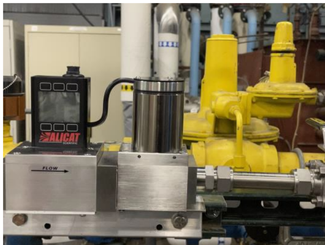
Installed H_2 flow meter for testing with higher H_2 and all parts ordered for assembly
