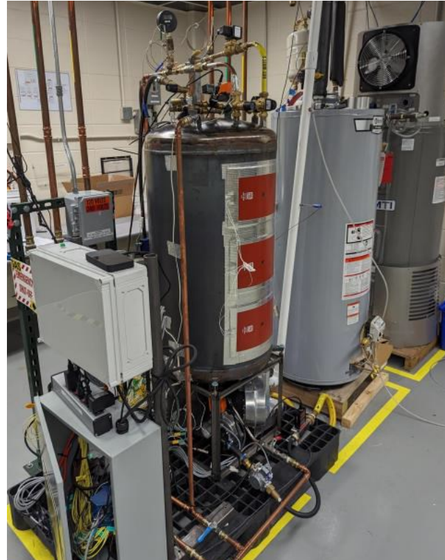
The "Alpha" Prototype Set-up for laboratory evaluation at full-fire.
