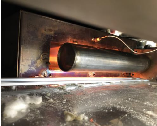
Left: Burner firing in the combustion chamber. Right: Premix burner installed on the bottom of an oven.
