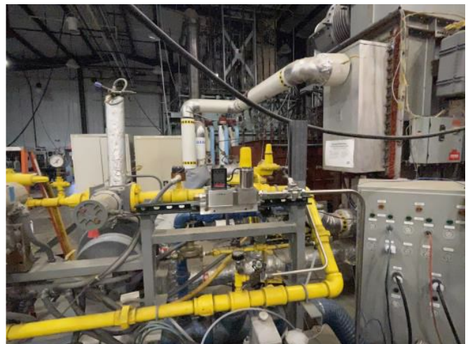
Installed H_2 flow meter for testing with higher H_2 and all parts ordered for assembly
