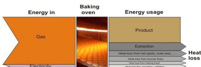
Energy input/output of traditional ribbon burners
