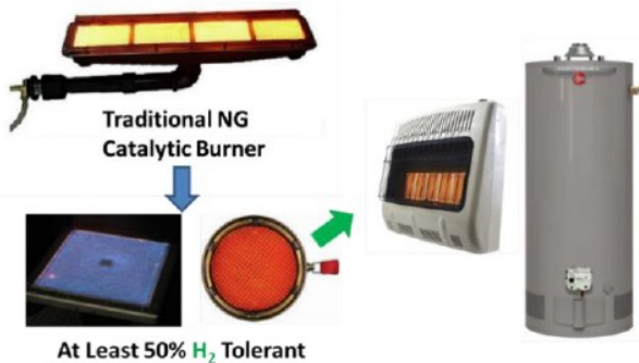
Improved Catalytic Burners can provide Fuel-flexible Operation
