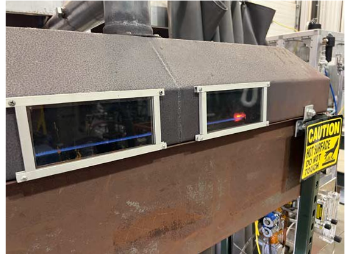
Ribbon burner test setup in laboratory
